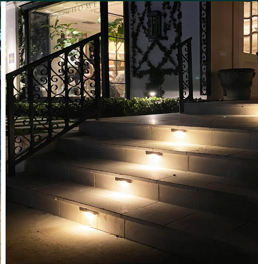
*Lite the Nite's* hardscape collection is an ingenious lighting option for projects involving decking, stairs, railings, walls, etc. built using just about any material - from wood, to brick, to stone. The slim profile allows for total concealment, yet provides a spray of light to brighten hardscapes.
